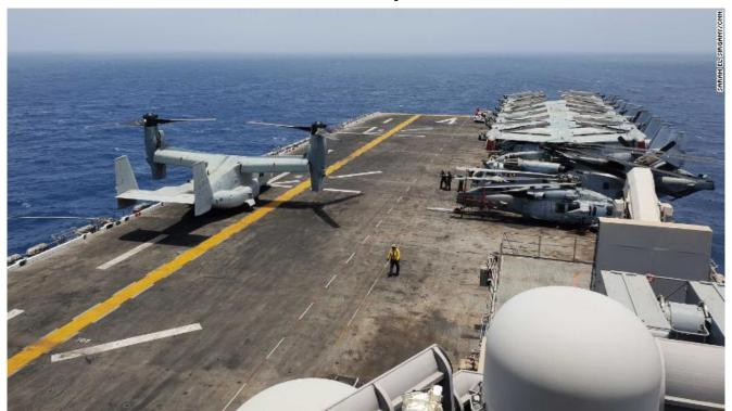
The USS Boxer's flight deck covers 2.2 acres. On the flight deck and inside its belly, the vessel carries the following aircraft: The Harrier, the Osprey, the Sea Hawk and the Sea Stallion.
